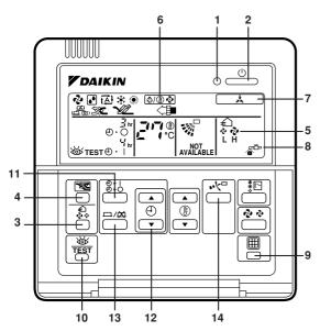
BRC1C51, 61, 517: Remote controller for VRV
